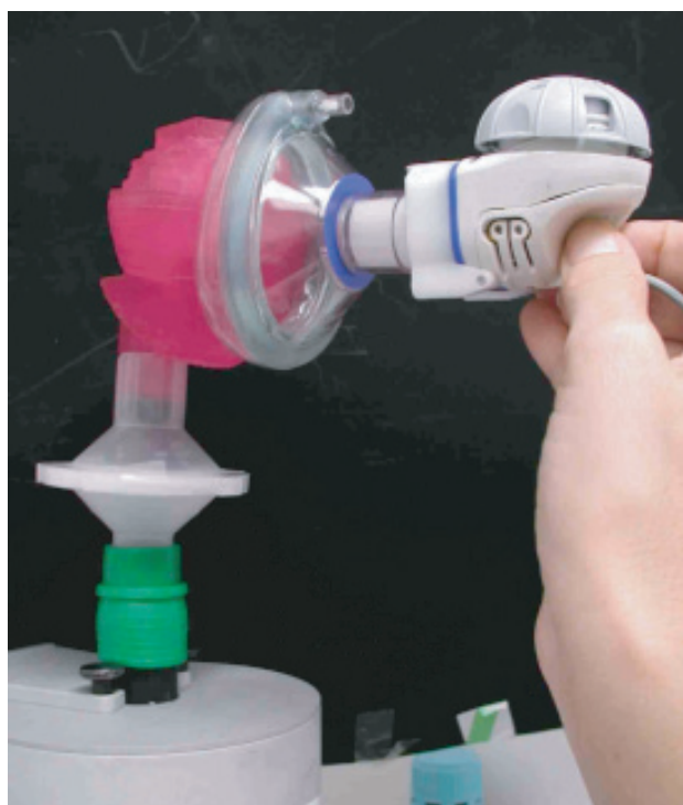
Figure 7. Test set-up to measure the aerosol distribution pattern using a baby cast. Used with permission from KELLER M, JAUERNIG J, SCHUEPP K et al. : Using infant deposition models to improve inhaler system design. Proceedings of the Respiratory Drug Delivery IX , Palm Desert, California, USA (2004):221-231.
